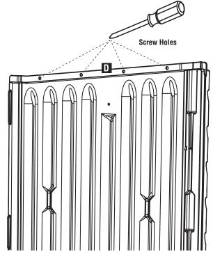
Connect Left Back (D) into dovetails of Repeat Left Side (C).
